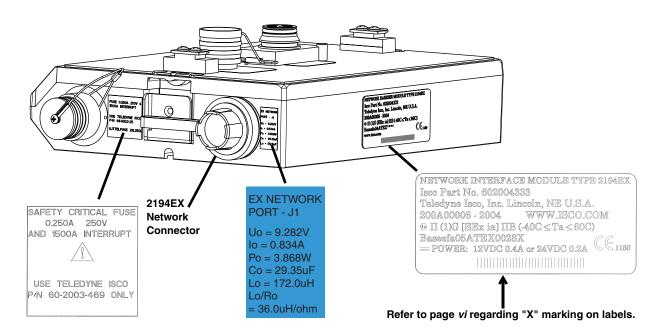
Figure 2-12 2194EX labels and cable connector
